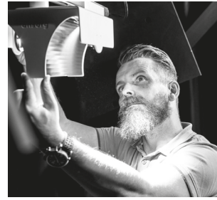
All developments are tested in the Ansorg Light Lab using a goniophotometer
